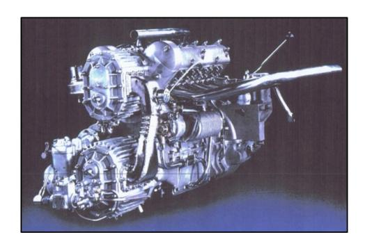
After 3 years of development, 9 months test on the dyno and a complete race season, we now have a reliable, high-performance engine for Maserati 4 CLT / 4 CL. The engine has about 260 real horse-power and high torque starting with low revs.
